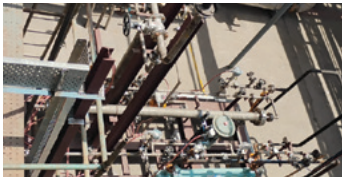
MTR membrane system for VC gas and N_2 gas separation.
